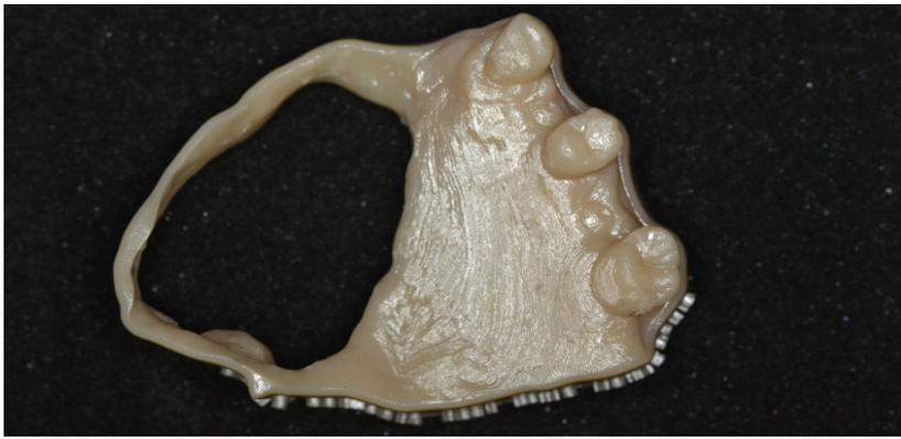
Fig. 6a. 3d printed maxillary cast
