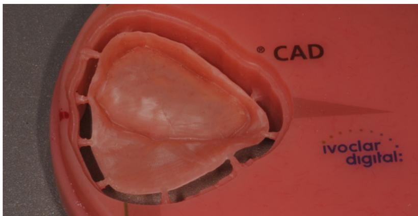
Fig. 8a. Obturator and denture base milled from Ivoclar CAD pink resin blank
