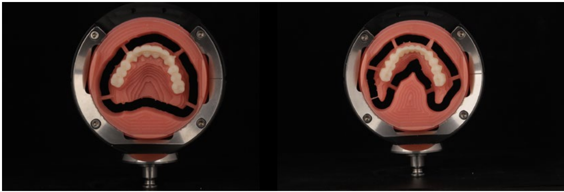
Figure 28 II. The oversized base and teeth polymerized and placed back into the PM7 for finalization.
