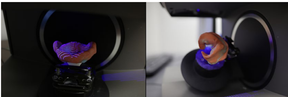
Figure 7. The maxillary and mandibular impressions are scanned utilizing the impression fixture in 3Shape (E Series) lab scanner.
