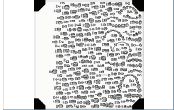
Automatic preparation for laser sintering.
